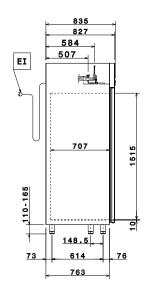
El = Electrical inlet (power) RI = Refrigerant Inlet = Refrigerant Outlet
